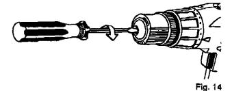
jaws securely. Tap sharply with a mallet in a counterclockwise direction. This will loosen chuck on the spindle. It can now be unscrewed by hand. See Figure 15.
